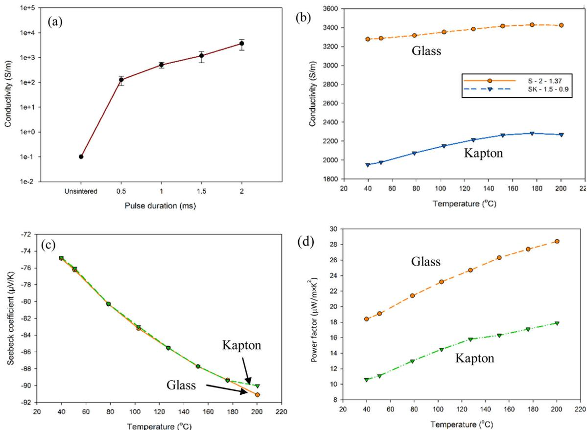
**Figure 2.** a) Electrical conductivity of the sintered samples by single pulse with increasing pulse duration from 0.5 to 2 milliseconds on glass. Temperature dependent (b) electrical conductivity (c) Seebeck coefficient (d) Power factor for the films on glass and Kapton substrate.
