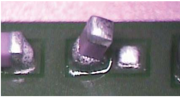
Fig. 1. Optical image and cross-section of a 0201 capacitor lifted after solder reflow [1].
